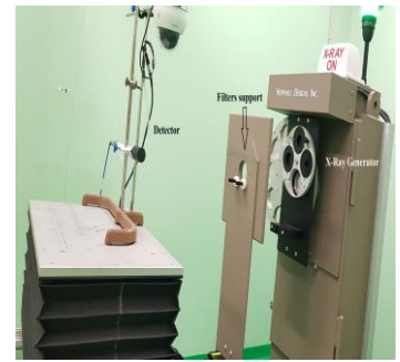
Figure 3: Experimental setup for half-value layer measurement
