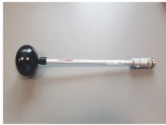
Figure 2: Ionisation chamber used
