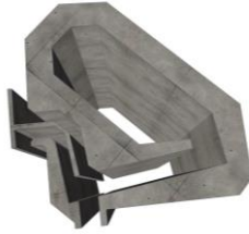
3D view of the source bunker
