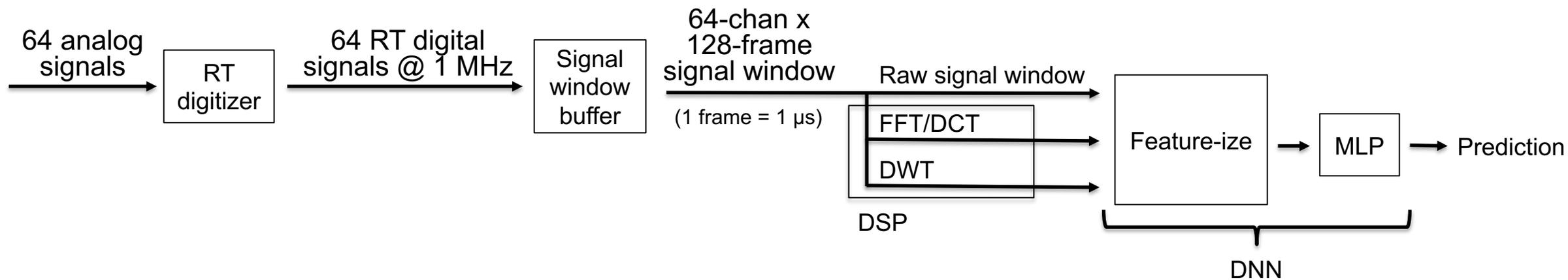
DNN must be compatible with high-throughput RT compute platform like FPGA
