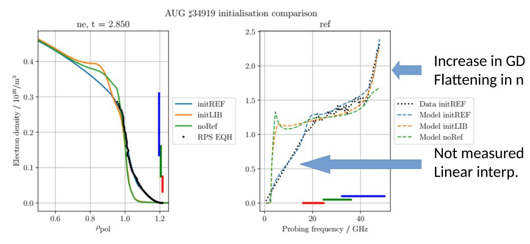
Measurement range in f and n: K-Band - Ka-Band - Q-Band
