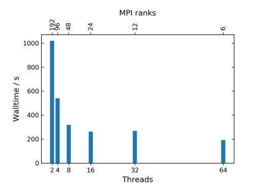
Run benchmark on 6 Cori nodes (Xeon Haswell CPU with 32 cores, 128GB RAM).
