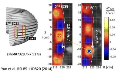
KSTAR ECE diagnostic: samples 24x8=192 channels with ~MHz sampling rate
