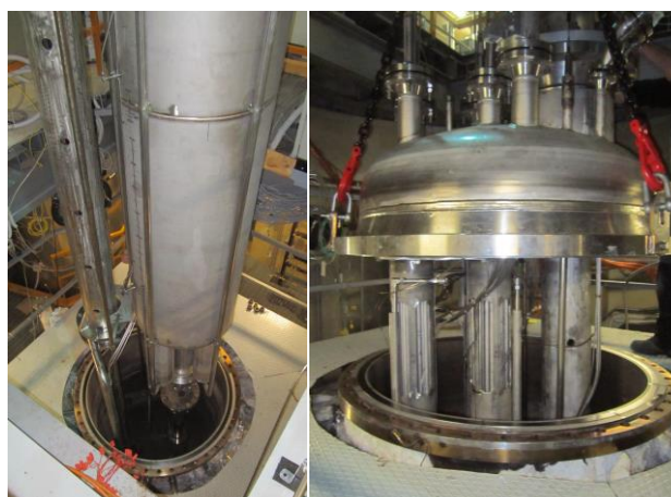
FIG. 15. CIRCE-SGTR test section.
