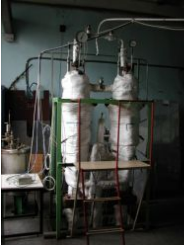
Experimental model for research of boiling in a system of parallel fuel assemblies
