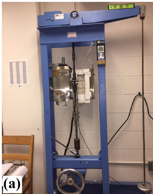
FIG.1 (a) Constant load lever arm creep machine. (b) Electrodynamic TestResources creep-fatigue machine (Model 810LE3) was employed for creep-fatigue tests
