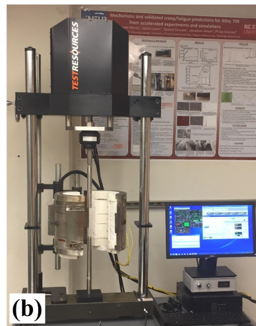
FIG.1 (a) Constant load lever arm creep machine. (b) Electrodynamic TestResources creep-fatigue machine (Model 810LE3) was employed for creep-fatigue tests
