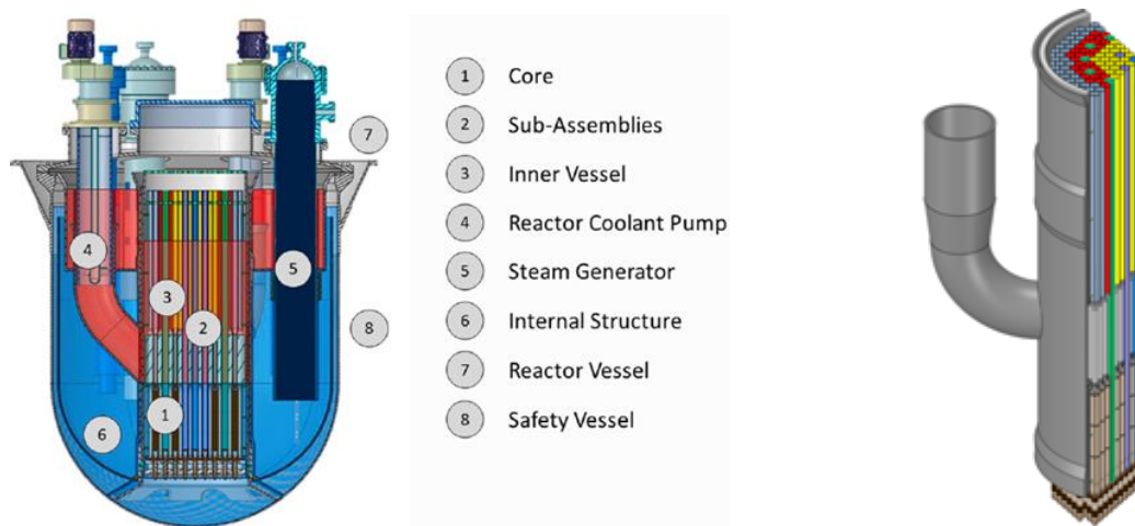
FIG. 1. Schematic drawing of the ALFRED reactor coolant system (left) and one symmetrical part of the ALFRED core with pump pipe (right).
