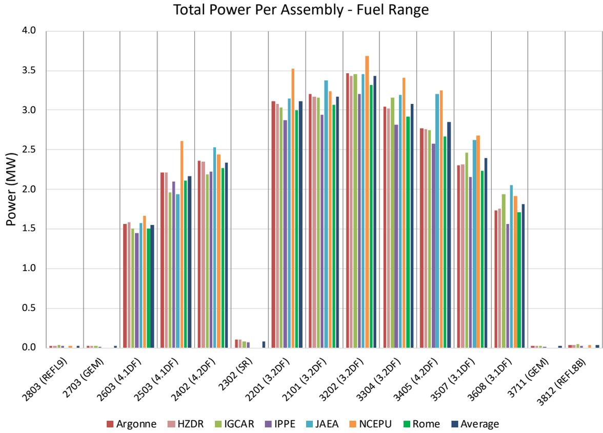
FIG. 3. Variation in Radial Power Profile In Several Assemblies
