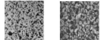
Microstructure of UN and U(Ce) N pellets
