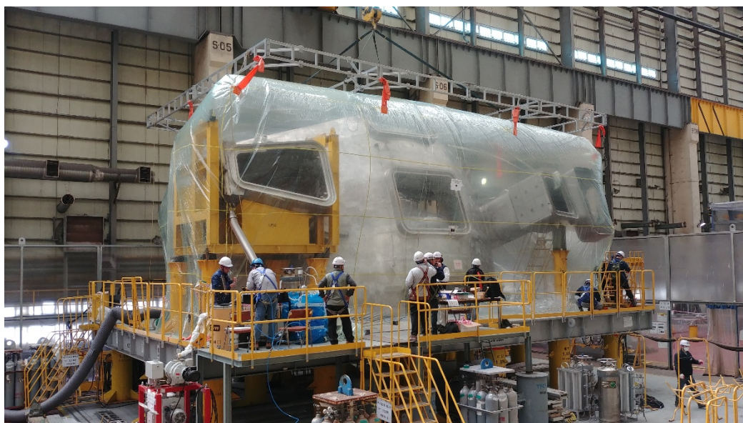
FIG. 8. He Leak Test of the ITER VV sector #6
