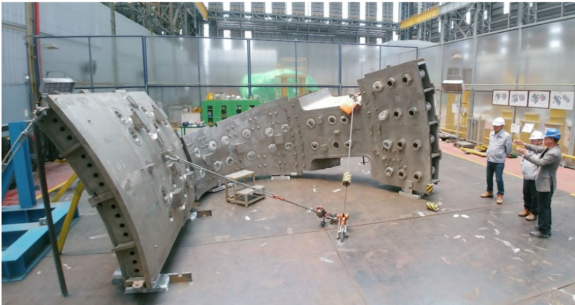
FIG. 2. Verification test of the precise handling technique using full scale PS1 and PS2 mock-ups
