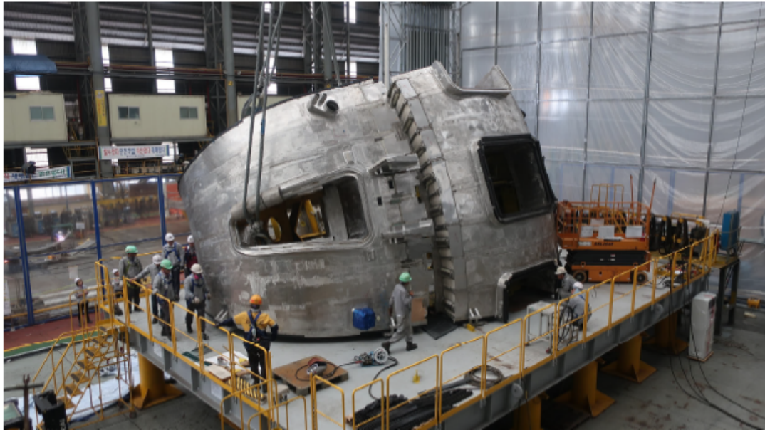
Figure 1: Final assembly of First sector at HHI on Aug. 2019
