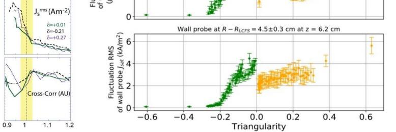
Reciprocating probe data showing particle flux, ion saturation current and cross phase between density and potential fluctuations. There is a large drop in the particle flux in the SOL in NT.
