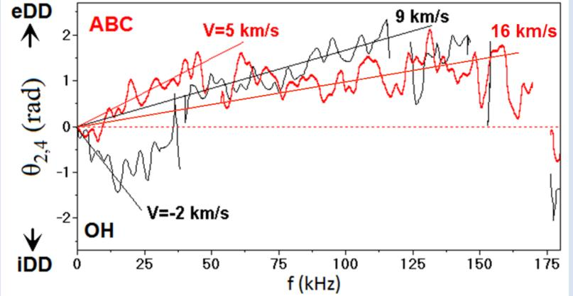
The cross-phase of density fluctuations vs frequency for OH (black curve) and ABC (red curve) stages of the shot with changes of the potential sign #73197;  $B_t = 2.2 \text{ T, } I_{pl} = 230 \text{ kA, } E_b = 320 \text{ keV, } r_{HIBP} = 0.09-0.11 \text{ m.}$
