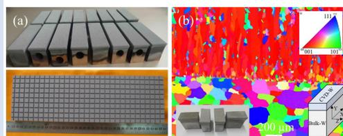
(a) large-scale CVD-W/CuCrZr mockups, (b) CVD-W deposited on Bulk-W substrate after heat treatment.
