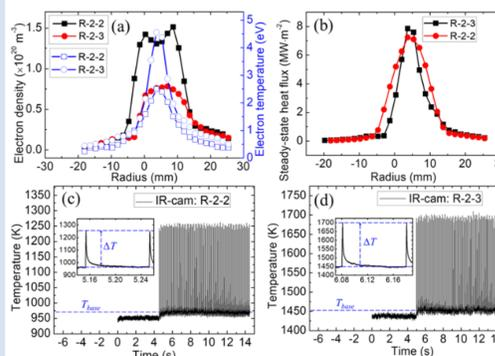
(a)  $n_e$  and  $T_e$ , (b) corresponding steady-state heat fluxes. (c) and (d) show the surface temperatures.
