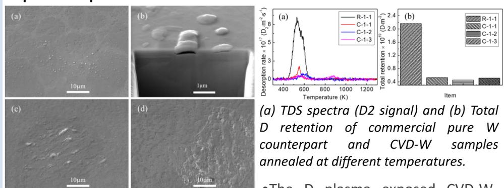
(a)/(b) The commercial pure W after D plasma exposure. (c)/(d) The exposed CVD-W annealed at 1273K/2373K.
