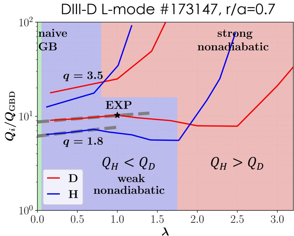
$$\frac{Q_i}{Q_{GBD}} = c_0 \sqrt{\frac{m_i}{m_D}} + c_1 q \mathcal{R} \sqrt{\frac{m_e}{m_D}} + c_2 (q \mathcal{R})^2 \frac{m_e}{\sqrt{m_i m_D}}$$
