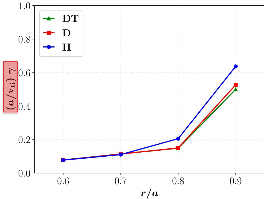
**Intrinsic Mass Scaling:**  $\gamma \sim \omega_{*i} \sim k_y \rho_i \frac{v_{ti}}{L_T} \sim \frac{1}{\sqrt{m_i}}$   $\rightarrow \left(\frac{a}{v_{ti}}\right) \gamma = \gamma_0$  independent of ion mass
