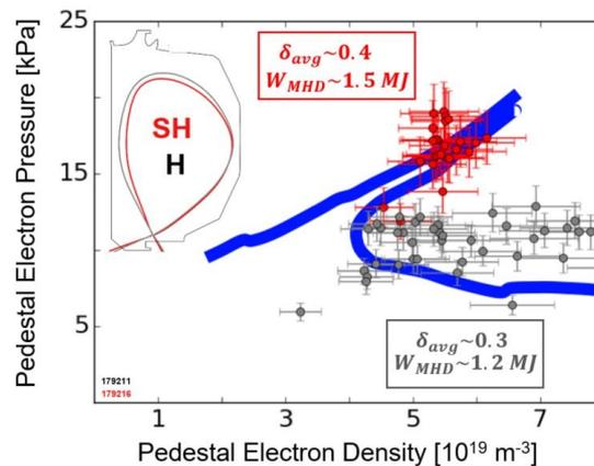
Figure 1: Density-pressure diagram showing Super H-mode channel access calculated from EPED for the  $\delta \sim 0.4$  discharge compared to DIII-D experimental data in two JET similar shapes. The higher triangularity shape (red) exhibits SH-mode operation, but the lower plasma shaping case (gray) does not.
