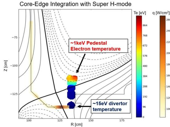
Figure 2: DIII-D divertor Thomson measurements in a Super H-mode with dual deuterium and nitrogen seeding. Pedestal temperatures are  $\sim 1\text{keV}$  and divertor temperatures are  $< 15\text{eV}$ . Infrared imaging heat flux measurements show reduced heat flux to the strike points due to  $N_2$  and  $D_2$  seeding.
