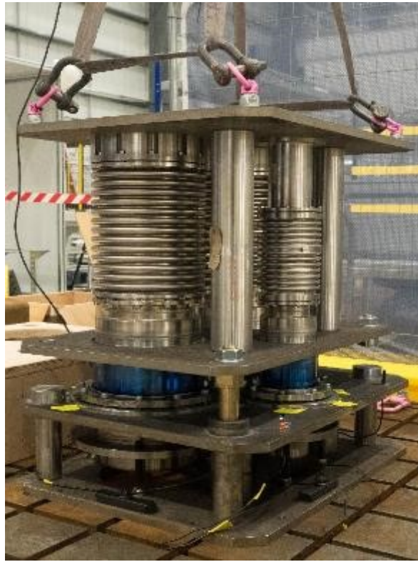
Figure 4: Testing the alignment of multiple pipes
