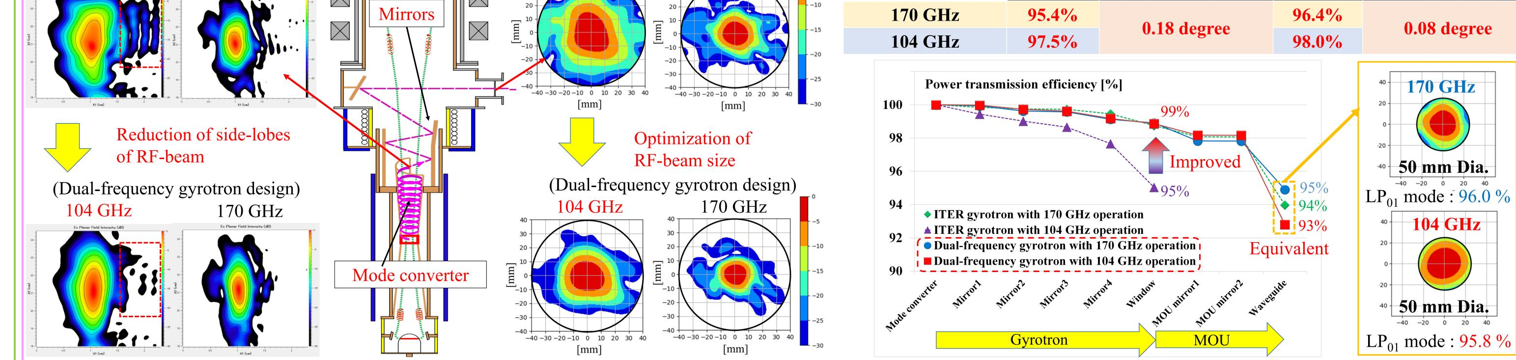
The side lobes of 104-GHz operation at the outlet of the mode convertor were successfully eliminated without affecting the beam pattern at 170-GHz operation. Moreover, the beam pattern for 104 GHz operation at the output window became smaller with minimal changes to the beam pattern at 170 GHz operation.
