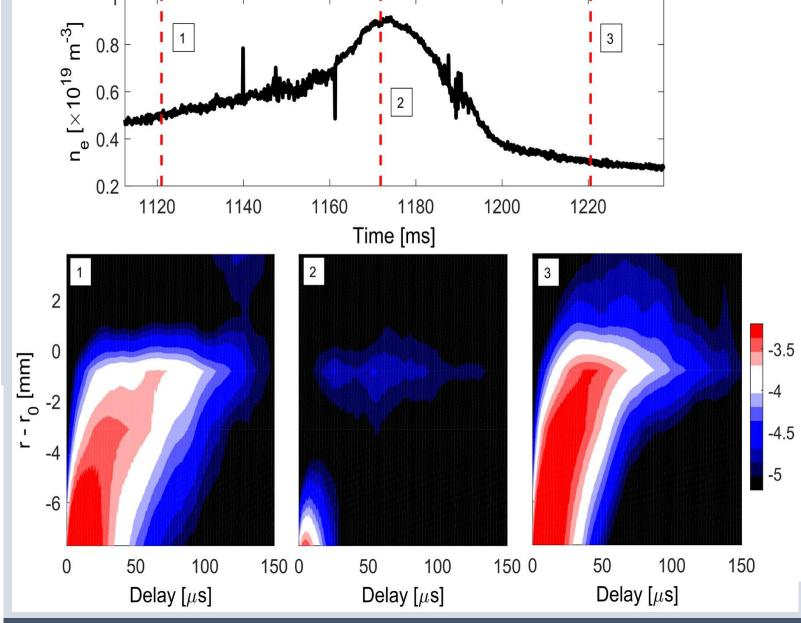
Turbulence radial spreading controlled by edge radial electric fields has been experimentally identified during the electron-ion root transition and edge biasing [Grenfell NF-2019 / NF-2020].
