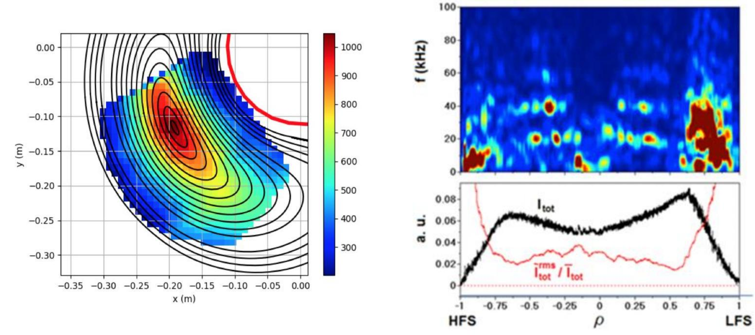
2-D mapping of plasma potential and density paves the way for model validation under positive and negative density gradient scenarios and asymmetries [Melnikov et al., EPS-2021].
