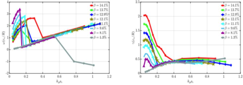
FIG. 5. Real frequency (a) and growth rates (b) versus binormal wavenumber of temperature gradient driven modes in the presence of energetic ions with  $\beta_f/\beta = 20\%$
