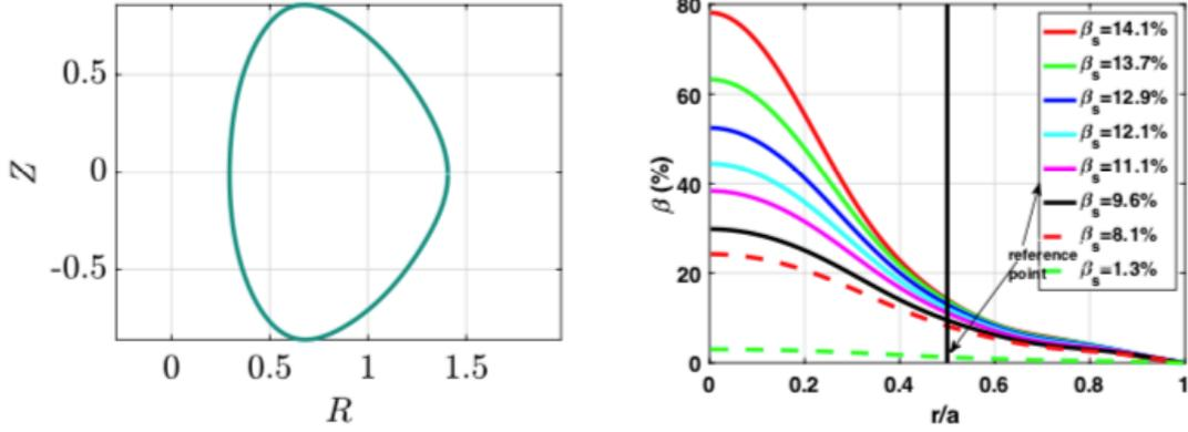
FIG. 1. Left: Shape of the last closed flux surface relevant to MAST and Right:  $\beta$  profiles for different equilibria. The values in the legend represent total  $\beta$  values at the location  $s = r/a = 0.5$
