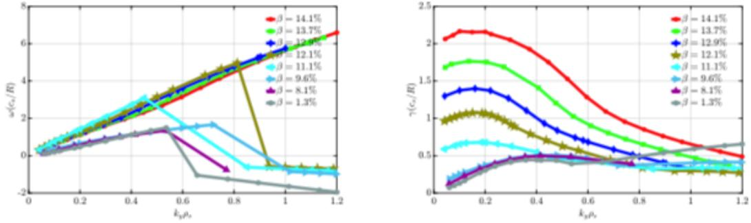
FIG. 3. Real frequencies (left) and growth rates (right) versus  $k_y \rho_s$  for the temperature gradient driven case, for two-species simulations.
