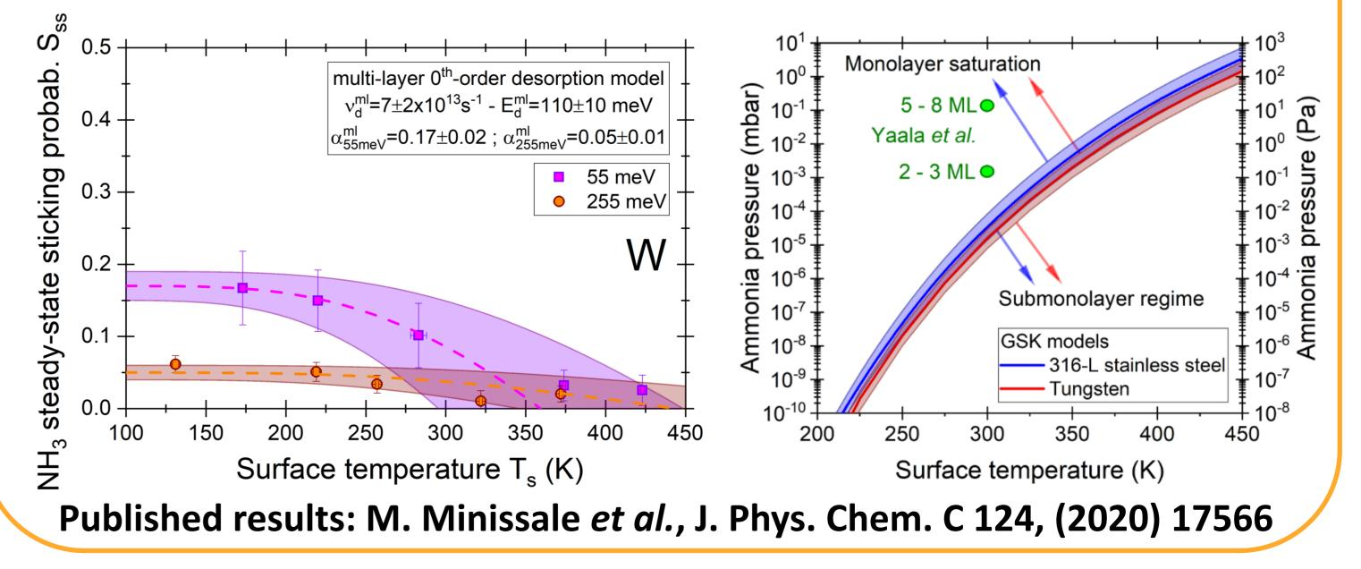
Conclusion Ammonia production is surface-limited on tungsten. Ammonia sticking on tungsten and 316L stainless steel is mediated by two precursors. Transient and steady-state surface coverage depend on NH<sub>3</sub> pressure and materials temperature and are described by the present models. The views and opinions expressed herein do not commit the ITER Organization in his role of nuclear operator.
