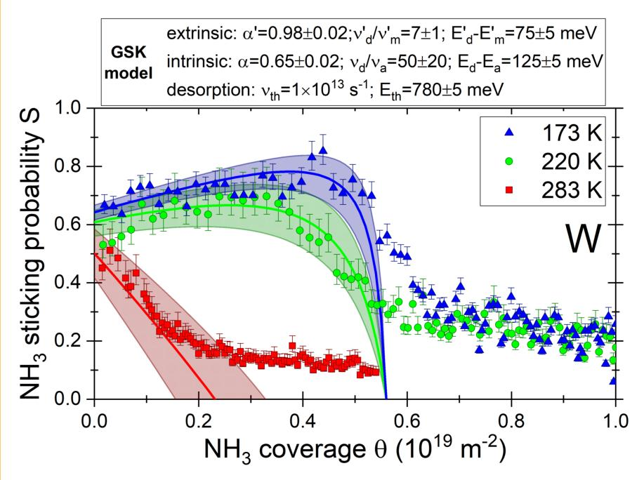
Α two precursors adsorption model & an island-based multilayers adsorption model are able to reproduce all our sticking results and are consistent with Yaala et al. (Nuc. Fusion 58 (2018) 106012) experiments
