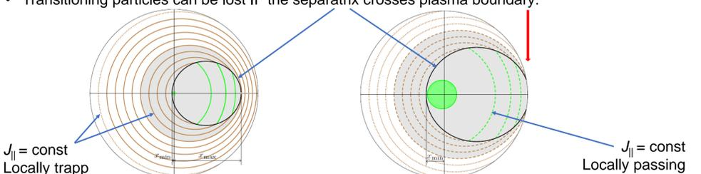
Bounce-averaged drift orbits (contours of  $J_{||}$ ) for locally trapped (brown) and locally passing (green) 3.5 MeV alpha particles in the intermediate Helias reactor (option "A") in the poloidal plane in flux coordinates. Left:  $\alpha = 0.12$ , right:  $\alpha = 0.15$
