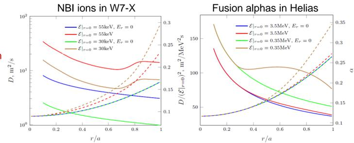
"intermediate" Helias, option A:  $R = 14\text{m}$ ,  $n_0 = 2 \cdot 10^{20} \text{m}^{-3}$ ,  $T_e \approx T_i = 10 \text{keV}$
