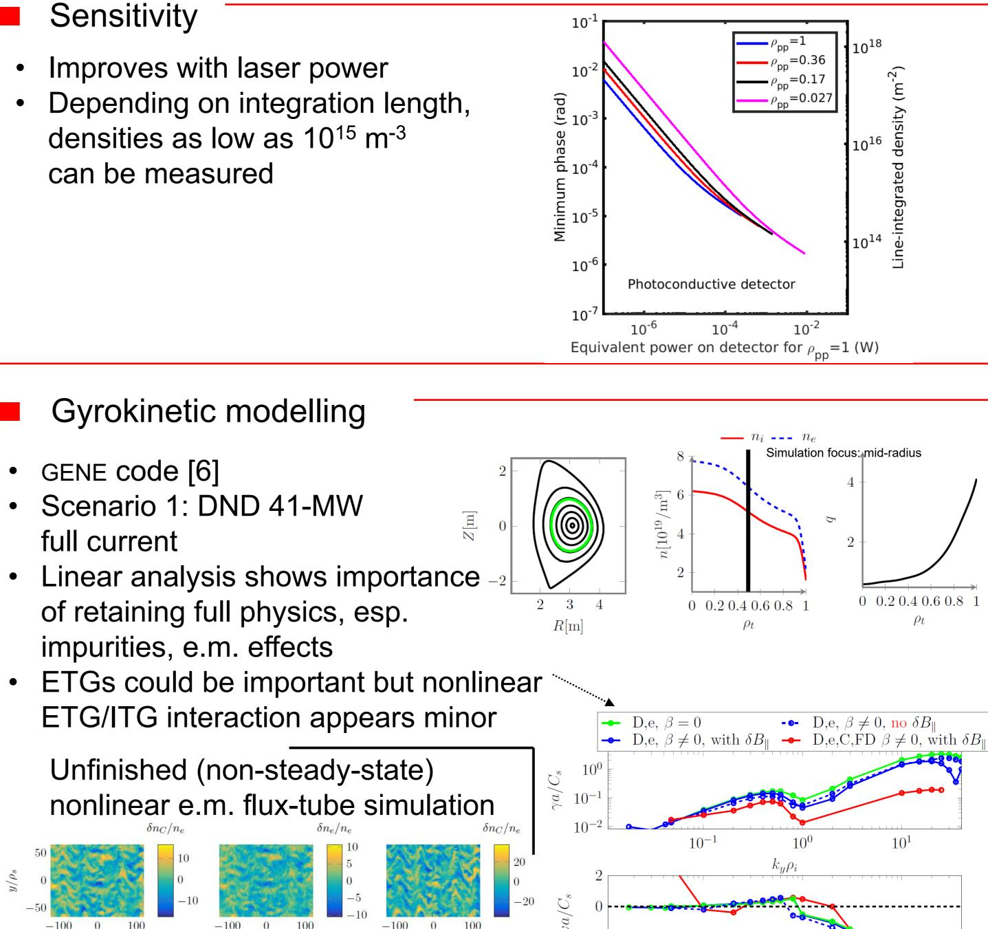
$\delta n/n \sim 10^{-5}$  sensitivity, in the range 0.06 <  $k\rho_i$  < 12 (potentially beyond: ITG/TEM/ETG), with high spatial resolution in the center and at the edge
