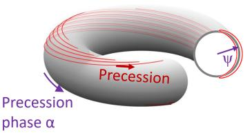
$$\frac{\partial f_s}{\partial t} + [J_0\phi, f_s]_{\alpha,\psi} + \omega_{d,s} \frac{\partial f_s}{\partial \alpha} = 0$$
