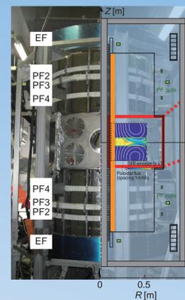
Magnetic flux surfaces with toroidal current density during merging ST formation in UTST
