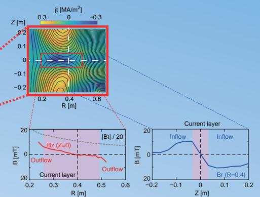
Toroidal magnetic field is about 20 times as large as the inflow magnetic field ( $B_r$ ).
