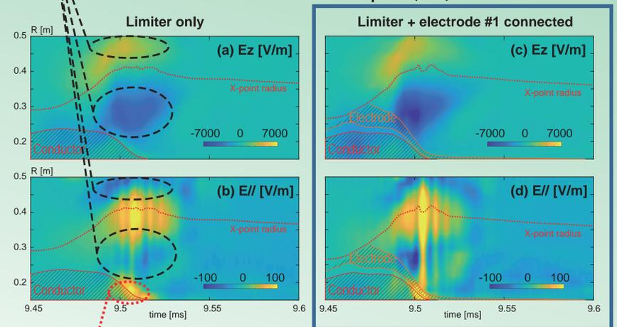
**inboard-side downstream region** : Parallel electric field survived where the field lines were connected to the limiter plate, which possibly suppresses the charge separation and reduces the axial electric field.
