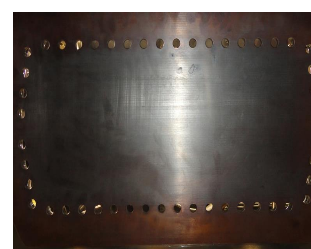
OFHC Copper Cooling plate after EB Test
