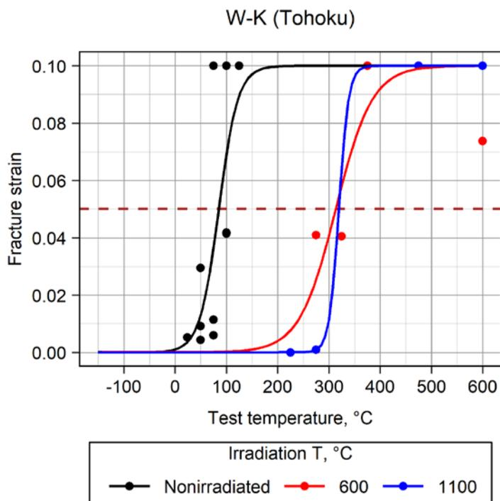
DBTT defined at the onset of flexural strain exceeding 5%
