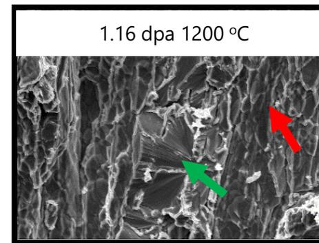
Red arrow: intergranular brittle fracture;
