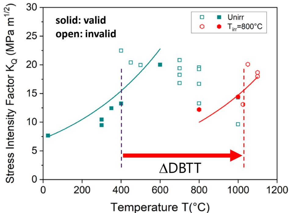
DBTT defined at the onset of **non-linear load-displacement** response
