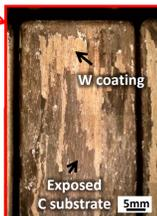
**Impact of arcs** lead to the delamination of the coating on the HFS of the tiles
