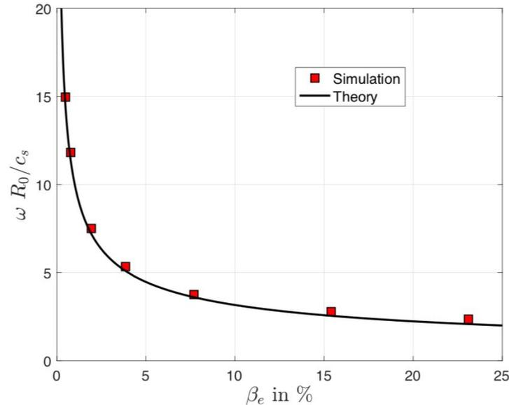
*Simulated and analytic real frequencies as a function of the electron plasma  $\beta$ .*
