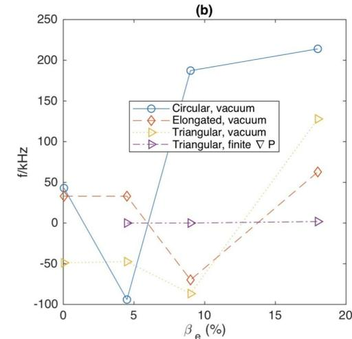
(a) Growth rates and (b) real frequencies as a function of electron plasma  $\beta$  for various compact toroidal geometries.
