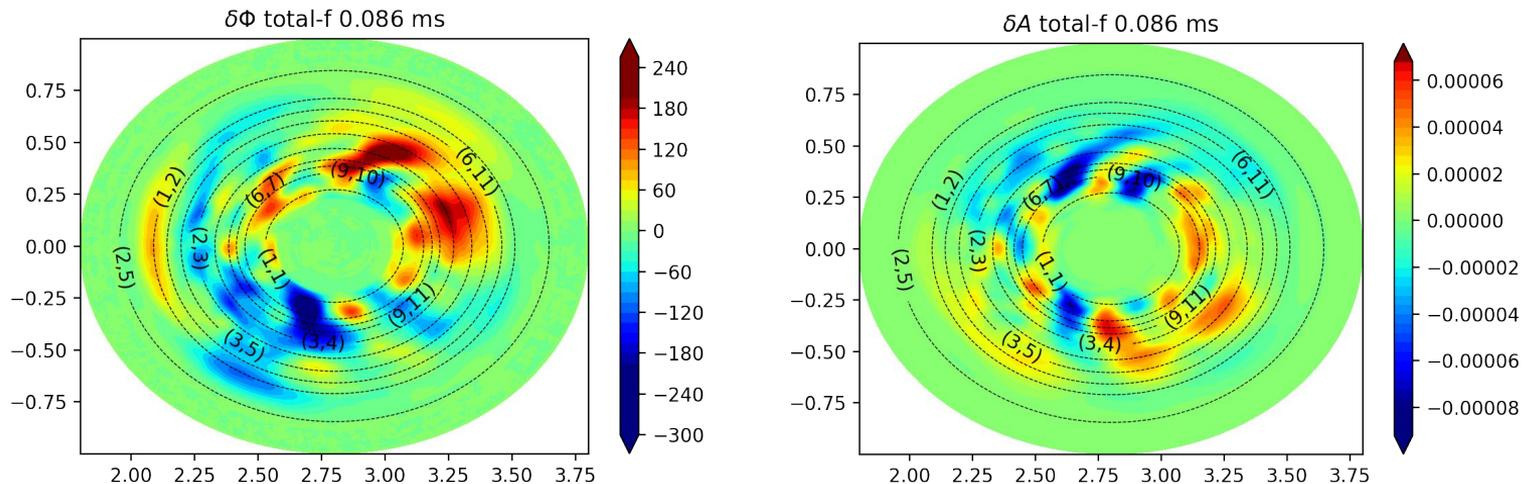
Electrostatic potential (left) and parallel magnetic vector potential (right) in the  $(R,z)$  plane at the KBM turbulence quasi-saturated state. Significant mode rational surfaces are indicated by dotted contours that are labelled with the resonant toroidal ( $n$ ) and poloidal ( $m$ ) mode numbers  $(n,m)$ .
