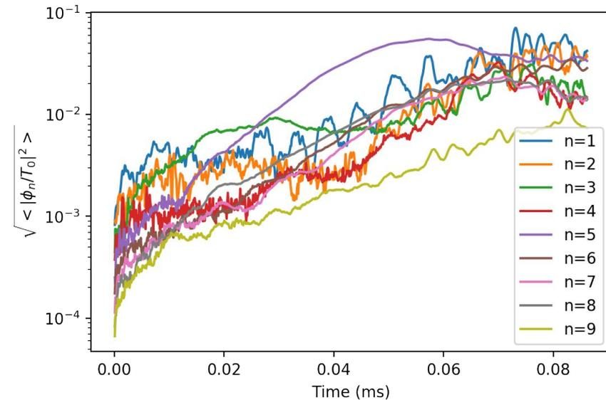
*Total-f explicit electromagnetic simulation in the ECBC tokamak plasma showing the electrostatic potential turbulence level as a function of time for all toroidal mode numbers  $n=\{1, \dots\}$ , with low- $n$  modes excited first. Similar quasi-saturation is found for magnetic perturbation modes.*
