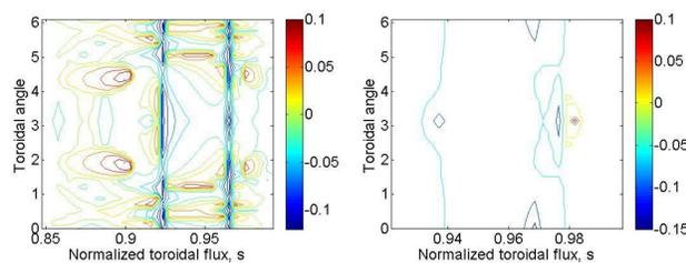
Figure 3: Contours of the ideal ballooning mode growth rate for (left) the current drive mode and (right) the 'external' or pressure driven mode.
