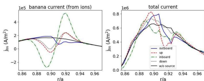
Figure 2: Scan of a) banana current and b) total bootstrap current as a function of radius for thermal particle source located at four different poloidal angles.
