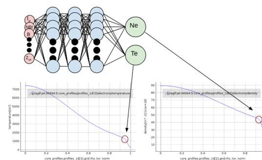
Figure 4: Illustration of how the neural network makes pedestal predictions from global parameters, and how the result is integrated in the European Transport Solver (ETS) to set new boundary conditions for the core transport models. Here, the profiles are taken from shot #96994 at JET
