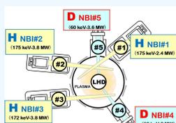
Fig. 2 Schematic of the LHD and the NBI systems.
