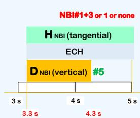
Fig. 8 Beam injection and plasma heating pattern.
