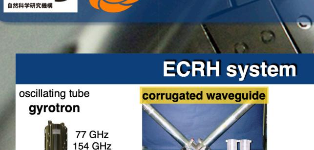
(LHD) **Electron Cyclotron Resonance Heating**
