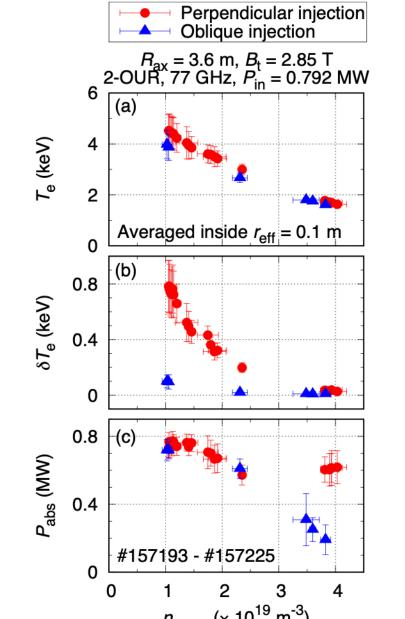
Absorbed power is higher by perp. injection for  $n_e > 3 \times 10^{19}$  m<sup>-3</sup>.
