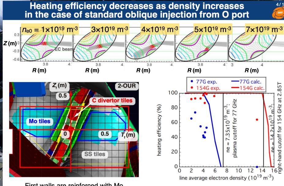
First walls are reinforced with Mo Effect of refraction mitigated on the opposite side of launchers. compared to injection from U port Contribution to ECCD experiments Courtesy of Y. Yoshimura
