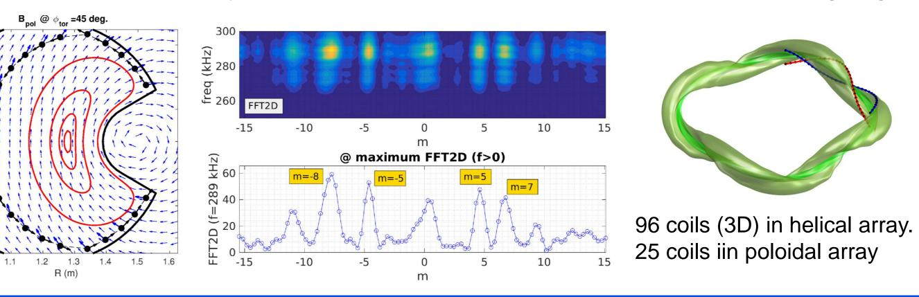
scenarios modifies the mode frequency. • FAR3d simulations accounting for changes in  $n_e(\rho)$  and  $T_e(\rho)$  and considering the combined effect on mode drive (higher damping (lower  $\eta \rightarrow$  higher an  $\beta_{fast}$ ) stability) predict a similar jump in frequency.
