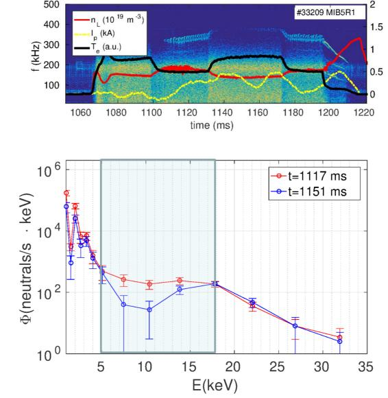
the result of the on-axis ECRH Similarly to experiment, a jump in mode frequency is again observed (with a larger change in density here)
