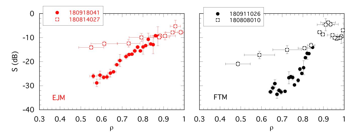
The density fluctuation level decreases from the plasma edge toward the core: the drop is more pronounced in the post-pellet phase than in reference puffing fuelled plasmas, and more in the high iota configuration than in the standard
