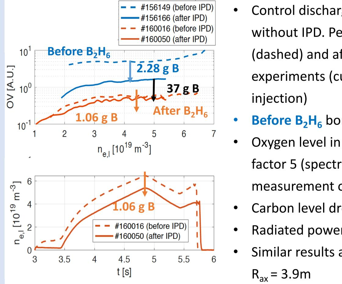
Control discharge: density ramp without IPD. Performed before (dashed) and after IPD
