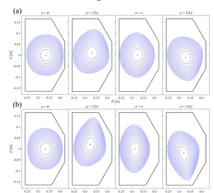
FIG. 10. Magnetic surfaces calculated with the condition of (a) FIG. 5, (b) FIG. 8
