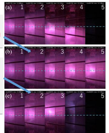
FIG. 6. Images of the plasma taken with a high-speed camera. The number displayed on the image means the time corresponding to the numbers in FIG. 5 (d). (a) w/o  $I_{SC}$  (b)  $I_{SC} = 2.6$  kAturn, (c)  $I_{SC} = 2.4$  kAturn with inverted current direction in side-installed SCs.
