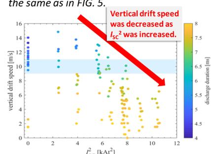
FIG. 9. Ensemble of vertical drift speed versus  $I_{SC}^2$  with discharges whose n-index were  $\sim -0.7$  and initial vertical position  $Z_p$  was  $1.0 \leq Z_p \leq 3.5$  cm.
