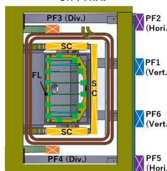
FIG. 2. Poloidal cross-section and coils of PHiX.
