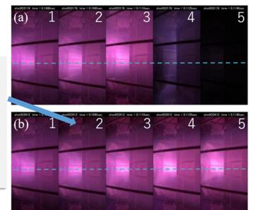
FIG. 8. Images of the plasma of tokamak discharges with divertor coils. (a) w/o  $I_{SC}$ , (b)  $I_{SC} = 4.9$  kAturn.
