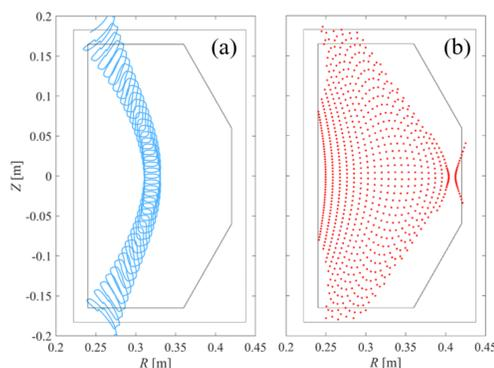
FIG. 3. (a) The magnetic field line projection of the poloidal plane, (b) the Poincaré plot of magnetic field line.
