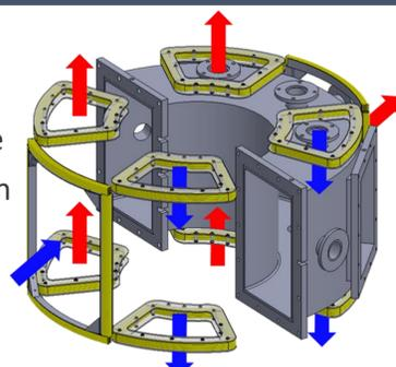
FIG. 1. Arrangement of SCs on PHiX.
