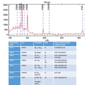
No prominent spectral lines was observed in the spectra after Y LBO obtained with the SOXMOS : a sea of small lines overlapping, for the most part, on similar ones from the intrinsic metals, presumably from Mo
