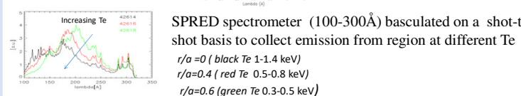
SPRED spectrometer (100-300 Å) basculated on a shot-to-shot basis to collect emission from region at different Te
