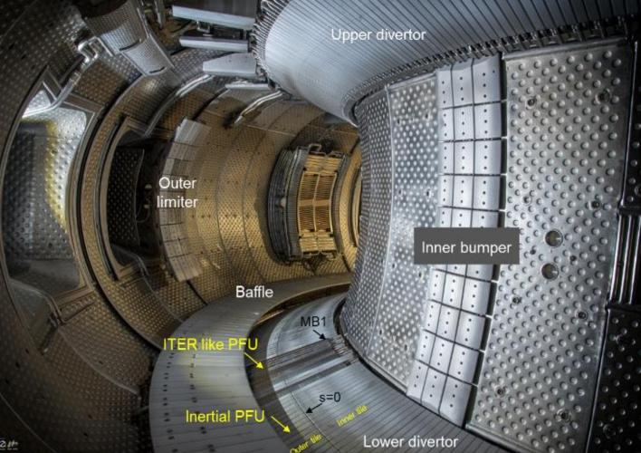
► WEST : a MA class superconducting device targeted at testing ITER tungsten divertor in a tokamak environment
