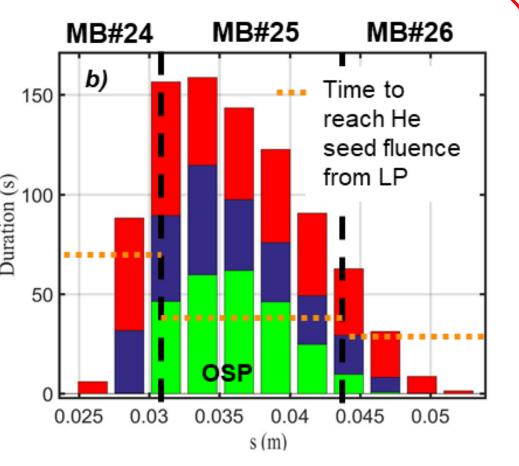
Fraction of He fluence impacting max OSP at Tsurf > 700°C only slightly above seed fluence (factor ~2)  $\rightarrow$  limited tungsten fuzz thickness
