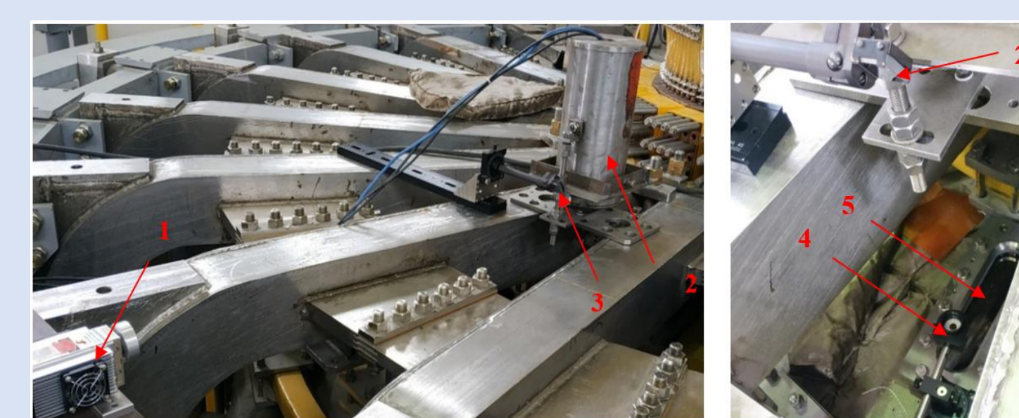
1-IR laser; 2-IR camera with magnetic shield; 3-rotary mirror; 4-homogenizer; 5-viewing window Equipment layout of thermographic measurements at the KTM tokamak
