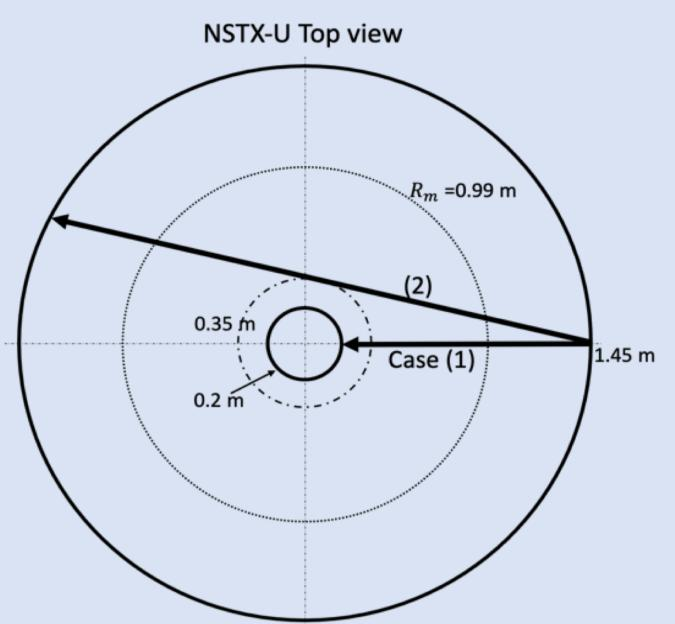
Top-down view showing the carbon pellet injection geometry. Case 1 is for pure radial injection, which minimizes the pellet propagation time to the magnetic axis. Case 2 is for a shallow injection cases, such as that which is likely to be used in the EPI configuration as in the absence of a plasma, the pellet could leave the vessel through a port at the opposite end of the pellet trajectory. This would avoid the pellet impacting the center stack of the tokamak.
