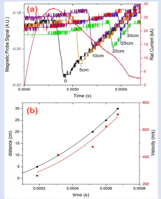
(Left)- Calculated parameters for near term tokamak test. With 4T boost magnetic field, velocities of 0.5 to 1km/s can be attained. (Right) -In a test of velocity potential using 2g sabot, 0.6 km/s was attained in < 1ms. The top right figure shows expanding magnetic field pulse behind the sabot as it moves along the accelerator. The bottom right plot shows distance traveled and velocity of the sabot as a function of time.
