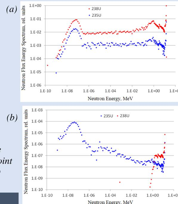
FIG. 5. Neutron spectrum (a) and the fission reaction rate (b) at the test point of IKD KNT 54-2-1 (238U) and IKD KNT-23 (235U).
