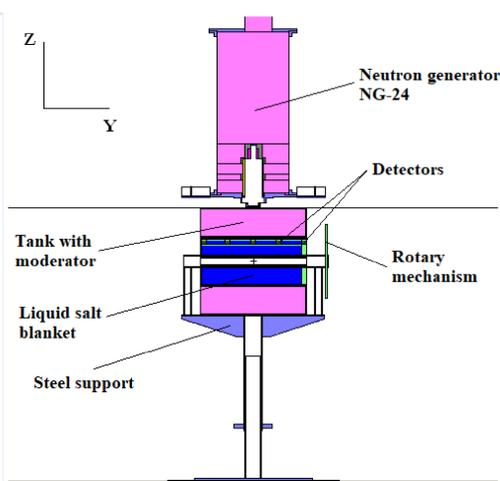
FIG. 2. Vertical section of a three-dimensional micromodel with the y-z plane.
