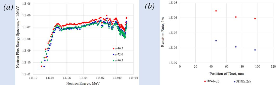
FIG. 3. Neutron flux energy spectrum (a) and the reaction rate (n, p) and (n, 2n) (b) in the blanket ducts located at a distance of r mm from the central axis of the blanket, when the duct with r=46.5 mm is in front of a 14 MeV neutron source with a power of 1 n/s.
