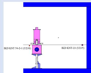
FIG. 4. Position of IKD KNT 54-2-1 (U238) and IKD KNT-23 (U235) detector in the experiment room.
