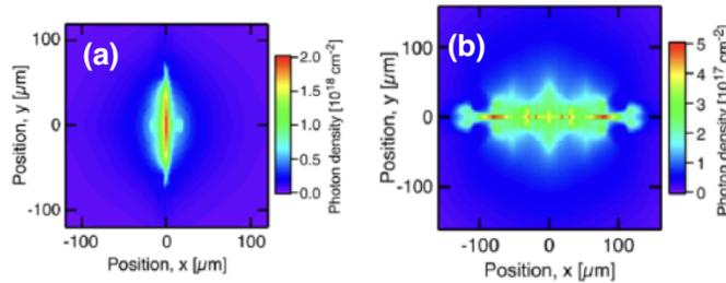
Figure 3: 2DSTAR-ALE simulation of GXII counter beams implosion at the maximum compression timing: (a) Temporal-integrated image of self-emission x-rays using a post processor for ray-tracing for Axial mode at 2.83 ns. Target is a simple CD shell. (b) Transverse mode at 2.86 ns. Target is a CD shell with two holes of 100  $\mu\text{m}$  diameter. The GXII peak is at 2.50 ns.
