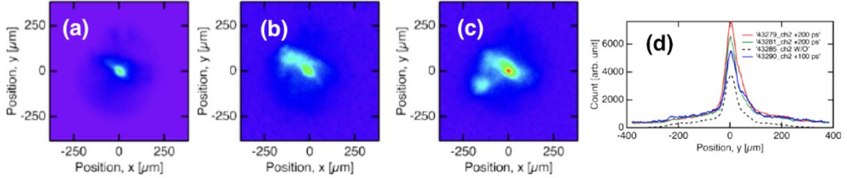
Figure 10: X-ray pinhole images of core (a)w/o LFEX, GXII 1.33 kJ (#4T3#43285), (b) LFEX 816 J at +100 ps, GXII 1.44 kJ (#5T4#43290), (c) LFEX 887 J at +200 ps, GXII 1.37 kJ (#3T2#43279); (d) x-axis scanned (a) dashed line, (b) blue line, and (c) red line.
