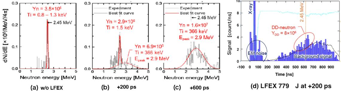
Figure 6: Neutron energy spectra from MANDALA (a) w/o LFEX #25T7#42488,  $Y_n = 3.47 \times 10^6/4\pi\text{sr}$  and  $T_i \leq 1$  keV for GXII energy of 1.65 kJ and (b) with LFEX of 261 J at +200 ps #24T3#42478, (c) with LFEX of 336 J +600 ps #24T2#42477. (d) Neutron time-of-flight signal with LFEX of 779 J +200 ps #4T1#43283 (at High power mode).  $Y_n = 8 \times 10^6/4\pi\text{sr}$ . [16, 17]
