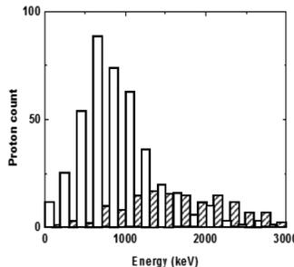
Figure 5: DD reacted-proton spectrum without LFEX from a track detector of  $0.4\text{ mm} \times 0.6\text{ mm}$ -square CR-39 films, positioned 5 cm far from the target. DD reaction has two branches, one of which yields n (2.45 MeV). Here, we use the another branch, yielding p (3.02 MeV). White columns are spectra shifted from 3.02 MeV along the transverse direction and striped are shifted to the axial direction, respectively[15, 14, 15].
