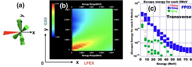
Figure 11: (a) Map direction: LFEX is on x-axis, GXIIs are up and down to y-axis(#5T4#43290). (b) Runaway electron distribution. (c) Electron spectrum: square is 21°, solid point 21°, and triangle 70° to x-axis, respectively. LFEX 794 J +200 ps (#3T4#43281 at High power) and GXII 1.44 kJ,
