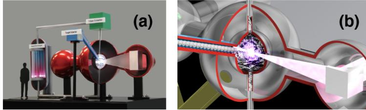
Figure 1: (a) Image of the Counter implosion fast ignition reactor CANDY. (b) Reactor chamber of CANDY[Movie:CANDY2015-English-0505-MPEG-4-1080-12000Kbps].
