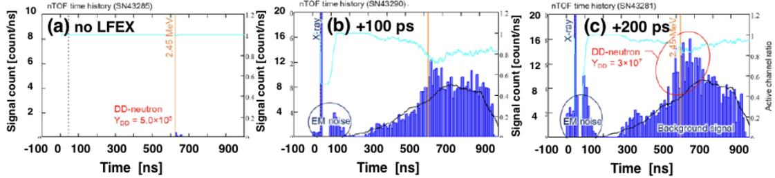
Figure 9: (a) No LFEX (#4T3#43285) GXII  $1.33\text{ kJ}$ ,  $Y_n = 5.0 \times 10^5/4\pi\text{sr}$ , (b) LFEX  $816\text{ J} + 100\text{ ps}$  (#5T4#43290) GXII  $1.43\text{ kJ}$ ,  $Y_n = 3.7 \times 10^7/4\pi\text{sr}$ , and (c) LFEX  $794\text{ J} + 200\text{ ps}$  (#3T4#43281) GXII  $1.44\text{ kJ}$ ,  $Y_n = 3 \times 10^7/4\pi\text{sr}$ .
