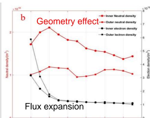
The density scan without impurity puffing is performed. The power flow to the inner and outer divertor keeps. The plasma density is found higher at LFS (due to the flux expansion), while the neutral density is higher at HFS (due to the geometry effect).
