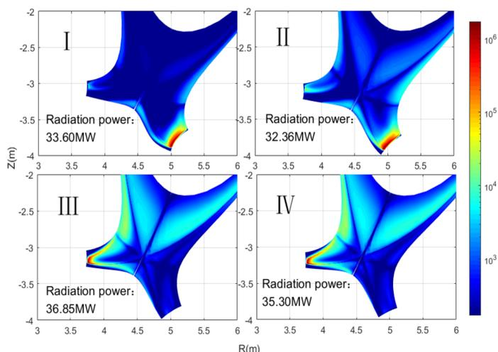
With the upstream density of  $\sim 2 \times 10^{19} \text{ m}^{-3}$ , the detachment is found in prior in LFS for the cases of larger flux expansion there, while the detachment can occur at the HFS in prior when the flux expansion is smaller.
