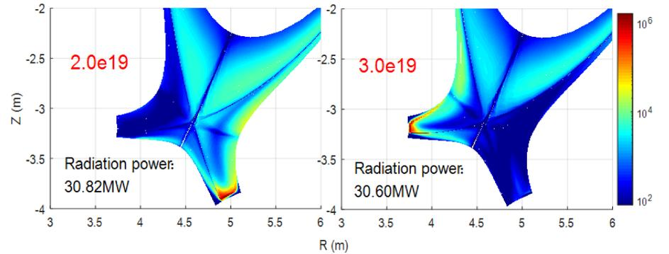
For the same configuration, the detachment occurs in prior at the LFS for low density, and at the HFS for high density.
