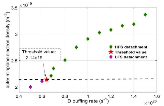
According to the density scan, it is found that the density threshold exists. The density threshold is found positively related to the flux expansion at the LFS.
