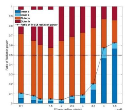
The DIVIMP simulation is performed by seeding Ne on the pure D background. It is found that the impurities is likely to stay at LFS for low density and at HFS for high density. With large flux expansion, the asymmetry of the impurity distribution is more obvious.
