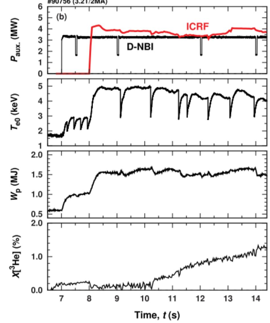
JET: D-(D<sub>NBI</sub>)-H scenario with fast NBI ions as resonant absorbers
