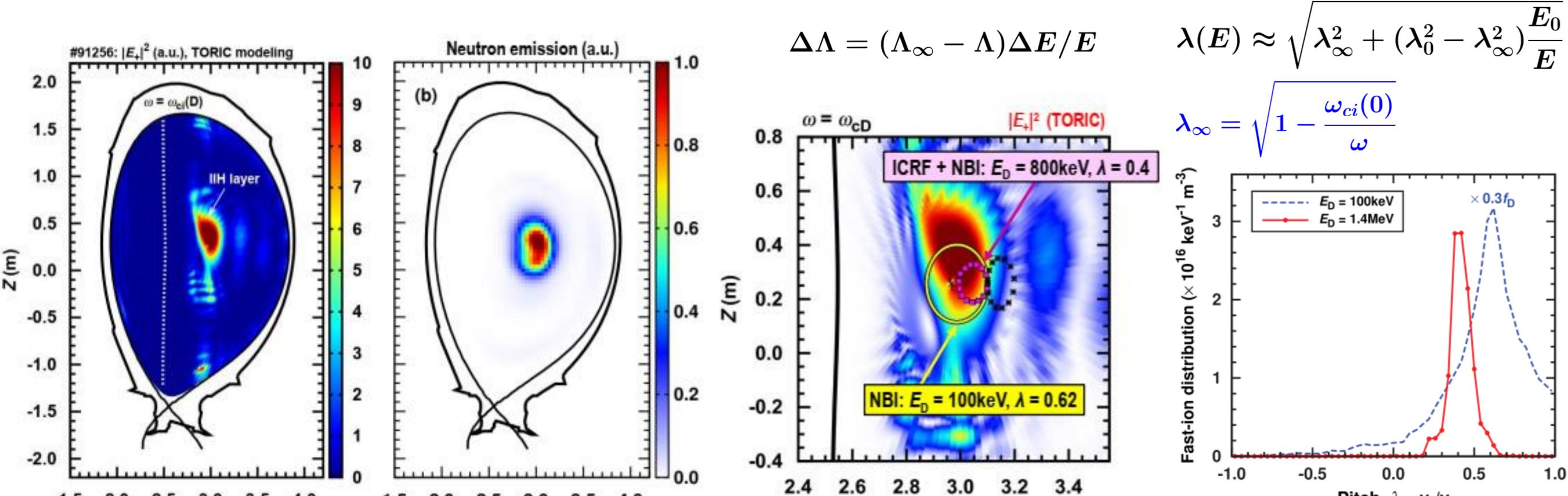
Asymmetry in  $k_{||}v_{||}$  → localized fast-ion current drive
