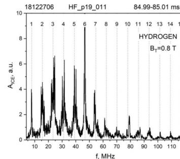
Fig.4. Ohmic ICE spectrum in shot with  $\bar{n}_e = 3.2\cdot 10^{19}$  m $^{-3}$  (#18122706), working gas – hydrogen. Probe location – 11° above equatorial plane in poloidal direction.
