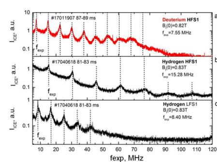
Fig.3. Ohmic ICE spectra measured in deuterium – a and hydrogen – b plasmas using probe HFS1 and in hydrogen plasma using probe LFS1 – c
