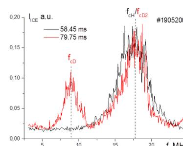
Fig.6. Ohmic ICE spectra obtained in hydrogen discharge before (black) and after (red) deuterium puffing
