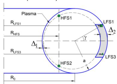
Fig.1. Projection of the probes location (green symbols) on poloidal cross-section, HFS1, HFS2 – probes locations at high toroidal magnetic field side, LFS1, LFS3 – probes locations at low field side,  $\gamma$  – poloidal angle, dashed line – plasma cross-section, grey area – limiter.
