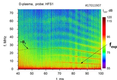
Fig.2. Ohmic ICE spectrogram in shot #17011907.  $f_{exp}$  matches IC resonance frequency in vicinity of the probe location
