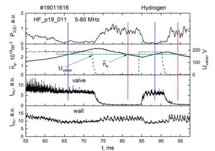
Fig.5. Evolution of the ICE power in the range of 5-80 MHz – frame 1,  $\bar{n}_e$  – frame 2, H-alpha Intensity in vicinity of puffing valve – frame 3 and far from valve – frame 4. Probe location – same as in Fig.4.
