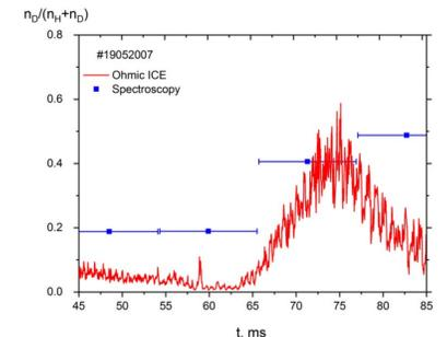
Fig.7. Evolution of  $n_D/(n_H+n_D)$  ratio obtained using intensities of ohmic ICE (red curve) and derived from H-beta/D-beta measurements (blue symbols)
