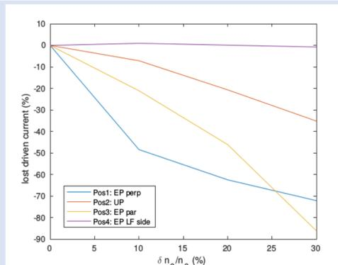
Figure 4: Lost driven current (relative to quiescent case) as a function of the perturbation amplitude. Large variations between launching configurations are observed.
