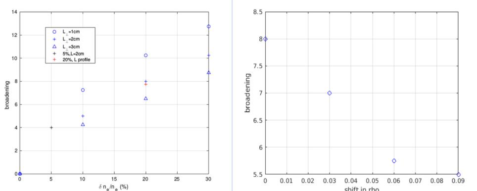
Figure 3: Broadening of the EC beam as a function of the fluctuation amplitude and correlation length for the position 1 (left). Broadening as a function of a shift of electron density profile (right).
