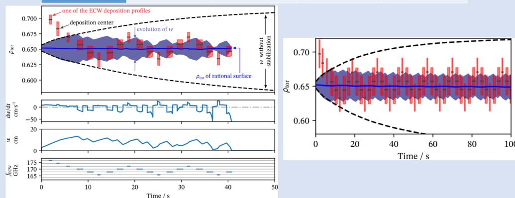
Figure 5: Mitigation of a NTM in the quiescent scenario (left) and the same assuming broadening by a factor of two, and power increase by x1.58 (19MW->30MW). Figure courtesy from Chuanren Wu.
