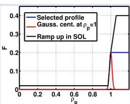
Figure 2: Profile of the fluctuation amplitude  $F=\delta n_e/n_e$  as a function of the radial coordinate. The blue profile is used in all simulations. Note that the amplitude of the core turbulence plays a minor role in these simulations.
