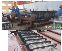
Frame to fix the inner & outer plate onto the surface plate. Target welding distortion:  $\pm 10\text{mm}$ .
