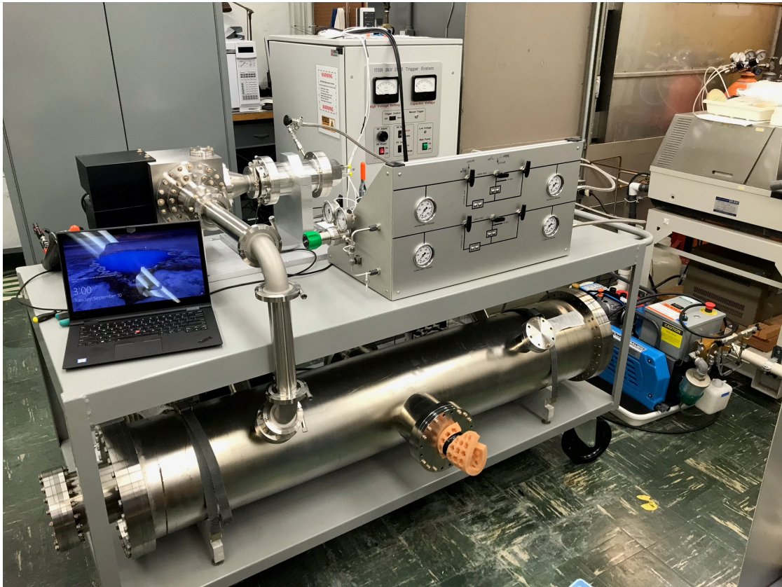
Figure 1: An image of the test set-up for the ITER relevant flyer plate valve without the external magnet.
